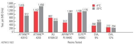
ATTANE<sup>™</sup> copolymers (especially ATTANE 4203) also retain superior toughness at low temperatures, as illustrated in Figures 4 and 5.
