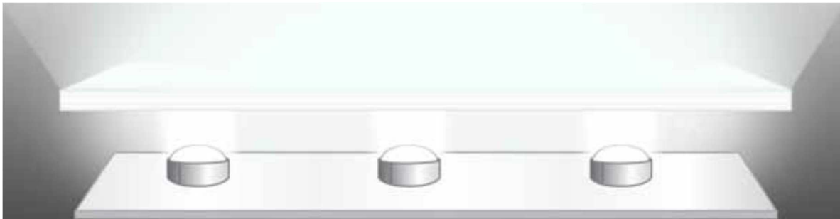
Transmission and Hiding Performance* of Plexiglas® Frosted and Diffuse™ Resins
