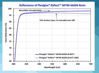
Extruded sheets from Plexiglas® Reflect™ MI7M-66204 resin blends provide a range of good to outstanding reflectivity in the visible light spectrum.
